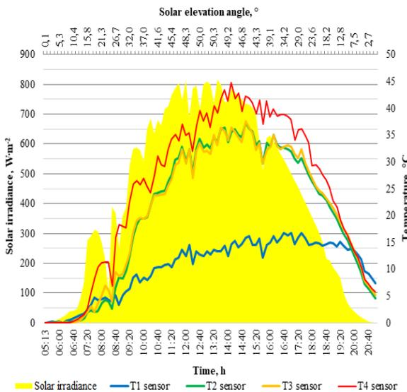
Fig. 9. Solar elevation angle, irradiance and temperature on May 8
