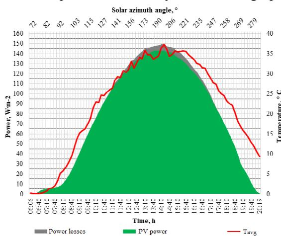
Fig. 10. Solar azimuth angle, PV power and power losses on April 16
