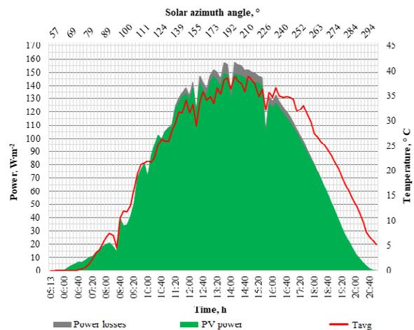
Fig. 13. Solar azimuth angle, PV power and power losses on May 8
