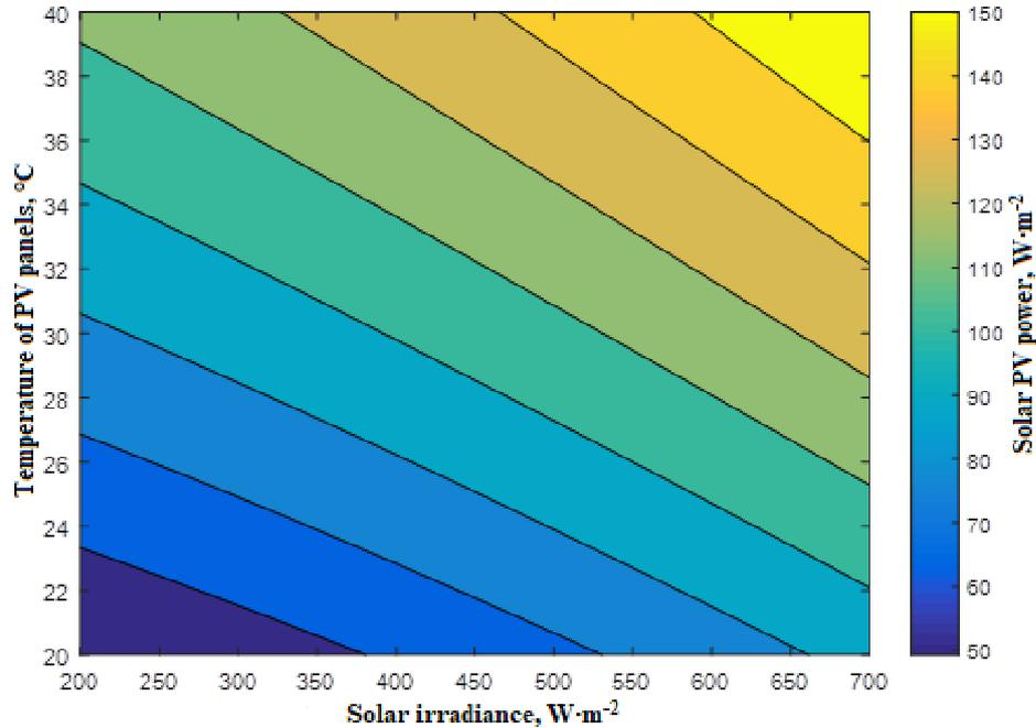
Fig. 14. Graphical interpretation of PV power, PV module temperature and solar irradiance
