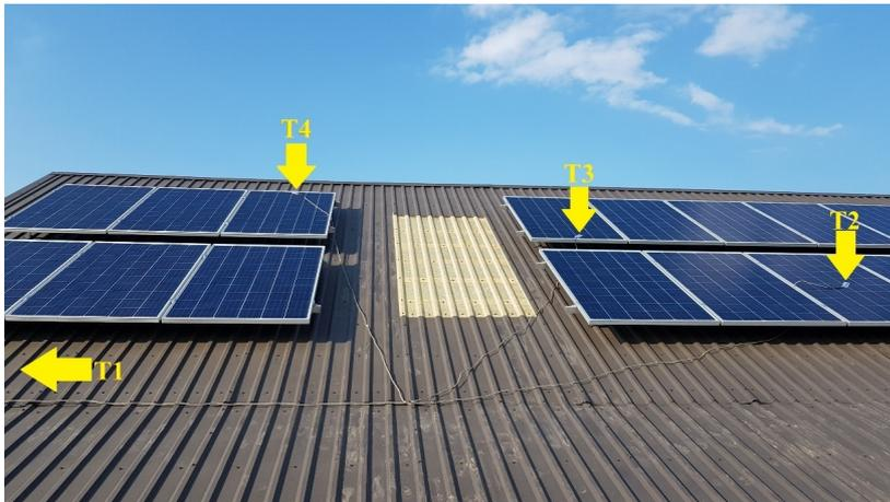
**Fig. 2. Placement of temperature sensors on PV modules:**
